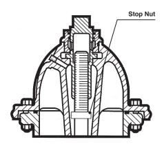
7. Turn operating nut in closing direction to make sure main valve is closed tightly, then turn in opening direction 1/4 turn to relieve tension on the operating mechanism.
