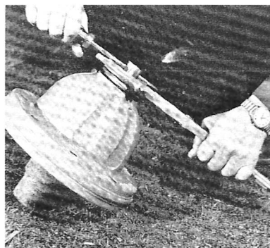
8. Place stop nut - operating nut assembly in bonnet. Place antifricition washer in bonnet. Thread in hold down nut making sure "O" - Rings are in place. Tighten hold down nut (recommended torque is 250 ft. lbs.).
