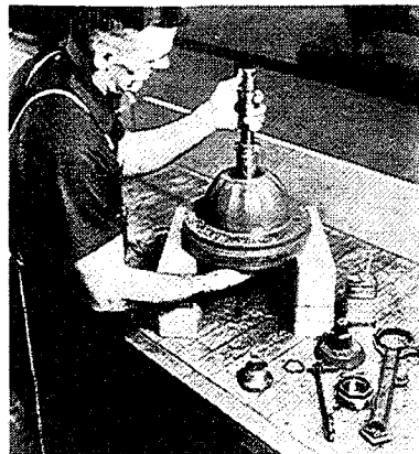
4. Remove and replace oil in stem nut. Fill stem nut with Mueller hydrant lubricant (approximately 2 oz. required) while part is setting level on bench. Oil level is to be even with oval slots in sides of the stem nut.
