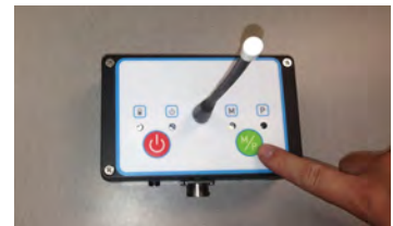
STEP 3: SELECT PIPE MATERIAL ON TRANSMITTERS.
