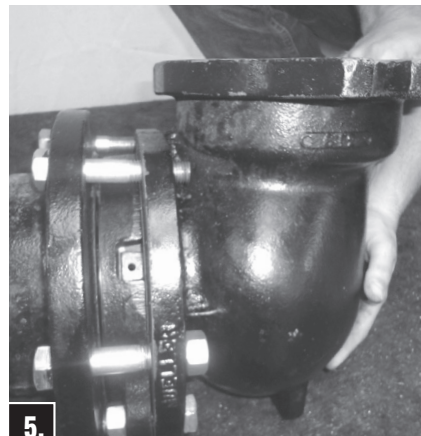
5. Slip new Shoe in place being careful not to damage Bottom Seat Ring O-ring.
